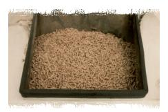
Pellets for domestic and small scale applications are typically 6-8 mm diameter, industrial applications are 10-12 mm.
