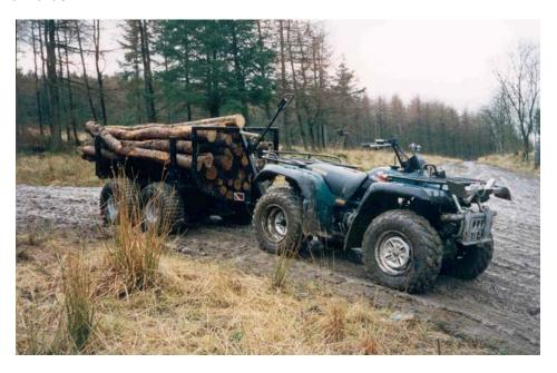
Comprises a 4WD ATC (>350cc) and a purpose-built trailer. Equipment need not be solely dedicated to timber extraction and is simple to set up and use. Cost ATC c. £6000, forwarding trailer £1800.
