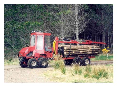
A purpose-built mini forwarder with 6 or 4 wheel drive. The narrow width of the machine enables working in closely spaced trees. The machine can be easily transported on a trailer towed by a 4WD vehicle. £26 500.
