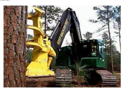
Cuts and accumulates several stems in the head before laying them for forwarder or grapple skidder uplift.  $220^{\circ}$  rotational head, cutting capacity 546 mm. Cost of head c. £15 000 – 20 000.
