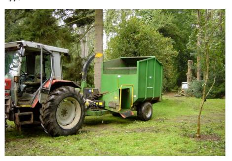
A trailer mounted NHS 720 chipper with a hopper coupled to a conventional agricultural tractor. Manually fed enabling collection of wood chips and transport out of wood. Cost £16 000.
