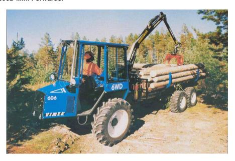
A 6-wheeled purpose-built machine with a loader reach of 4.2 m, capable of carrying 3000 kg. The low ground impact ability of the machine makes it suitable for woodlands with a weak soil structure. Cost £39 550
