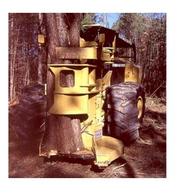
Harvester with a 16-tooth single piece cutting disc. Ideal for small diameter thinning. Offset tooth design generates 2 1/4" kerf. Widely used in the USA.
