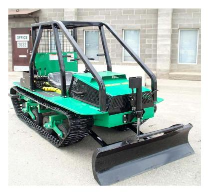
A Canadian machine with hydrostatic traction. Fitted with a winch it is capable of skidding tree lengths using a main line and chokers. Weighing 1250 kg and having an overall length of 2.41 m it can be easily transported using a 4WD vehicle and trailer. Cost c £16 500.
