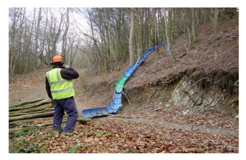
A series of connecting semicircular plastic lengths (4.2m) used for extracting small round wood, gravity fed and very useful in woodlands where access is restricted. Cost £50 per section.
