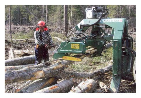
Attached to the 3 point linkage and hydraulic system of a conventional agricultural tractor. Loading can be by winch or grapple. Can cross cut logs up to 18 cm diameter. Cost c. £15 000.
