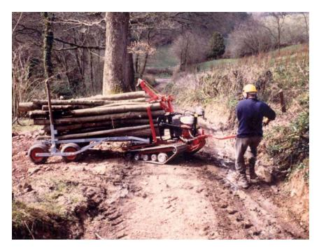
A pedestrian-controlled tractor with tracks, which can be used as a skidder making use of the integral winch, or a forwarder using a trailer. Versatile and compact with excellent terrain capabilities. Cost £8500 excluding forwarding trailer.
