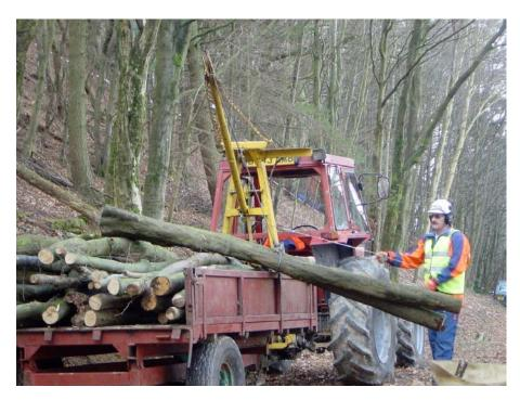
An 'A' frame incorporating a PTO driven winch and loading arm. The winch is controlled by a caddy line held in a cassette on the operator's back. Timber is extracted to the trailer using a skid cone. Cost £2345.
