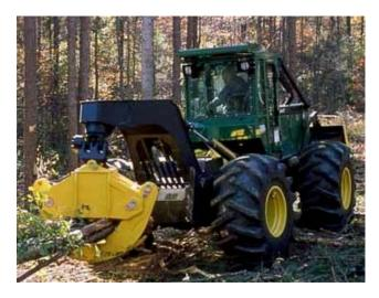
A 4WD single grapple skidder with exceptional manoeuvring capabilities. Potential use in a wood fuel production system with a feller buncher harvester
