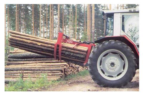
A triple jaw skidder with slewing cylinder coupled to the 3-point linkage of an agricultural tractor. Presentation of produce is important for efficient operation. Relatively inexpensive understated piece of extraction equipment. Cost £1610.
