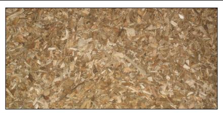
Sampling was carried out in accordance with the technical specification CEN /TS 14778 – 1: 2005 Solid Biofuels sampling. The sampled material was sent to an accredited sampling laboratory for particle size analysis. The standard specifications met by chips produced by the various chippers are shown in the table below:
