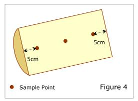
To measure the moisture content of a firewood log using a resistance type hand held moisture meter, it must be freshly split and then three measurements taken on the freshly split surface: 5cm in from each end of the log and in the middle of the split surface with sufficient contact (see figure 4). It is recommended that you test at least 5 logs from each 2m³ batch. You should then calculate the average (mean) MC over all of the readings.
