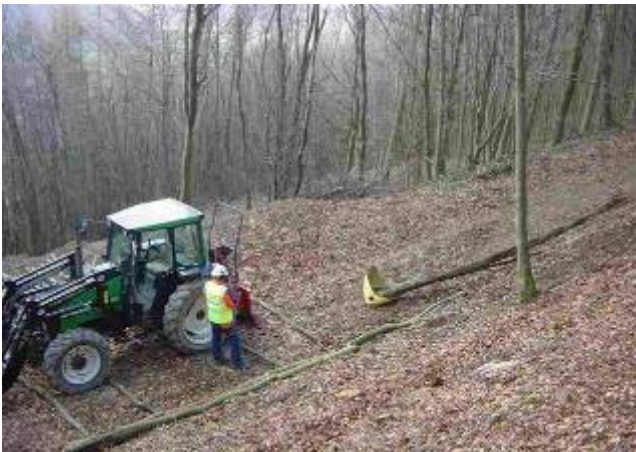
Figure 11 Modified agricultural tractor skidding pole length produce on steep terrain Figure 12 Farm forwarder based shortwood extraction
