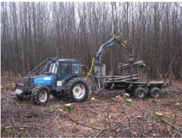
Figure 1 Medium Farm Forwarder 8 tonne un-laden weight
