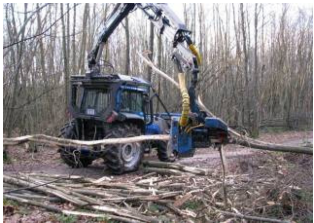
Figure 7 Valtra T160 with Keto 51 felling head harvester Configuration in Sweet Chestnut coppice felling Figure 8 Valtra harvester in Sweet Chestnut coppice felling
