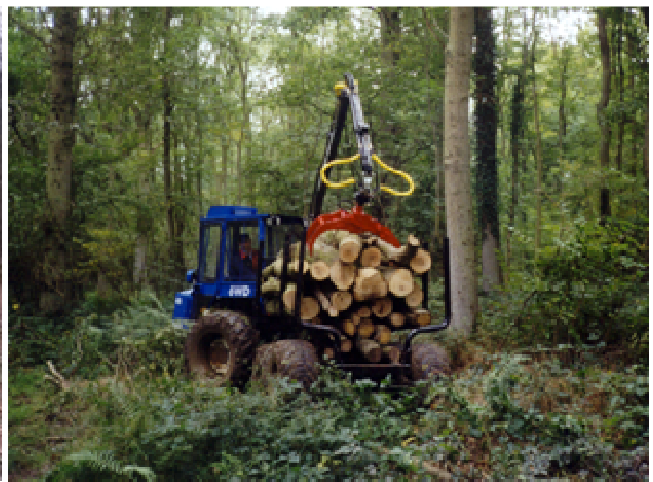
Figure 2 Vimek 606 Forwarder 3 tonne un-laden weight
