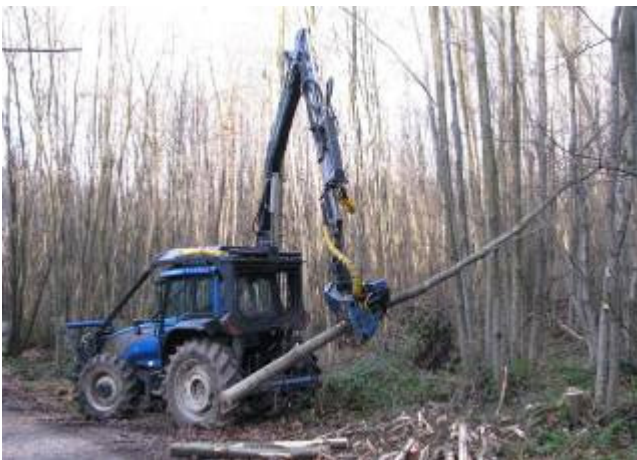
Figure 7 Valtra T160 with Keto 51 felling head harvester Configuration in Sweet Chestnut coppice felling Figure 8 Valtra harvester in Sweet Chestnut coppice felling
