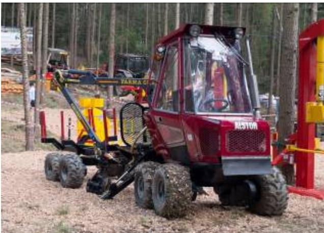
Figure 3 Alstor 831 Forwarder 2 tonne un-laden weight
