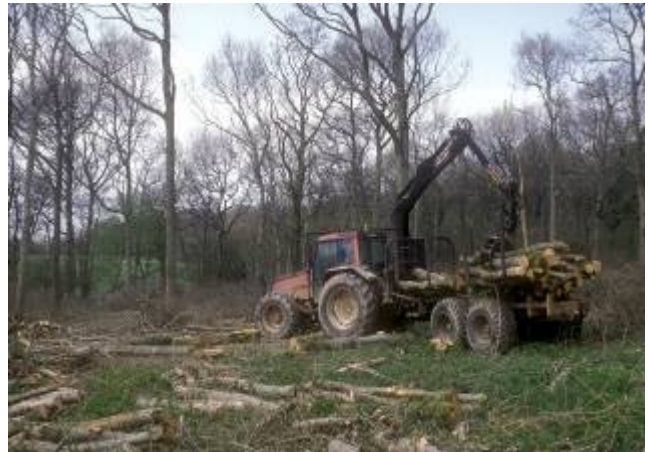
Figure 11 Modified agricultural tractor skidding pole length produce on steep terrain Figure 12 Farm forwarder based shortwood extraction
