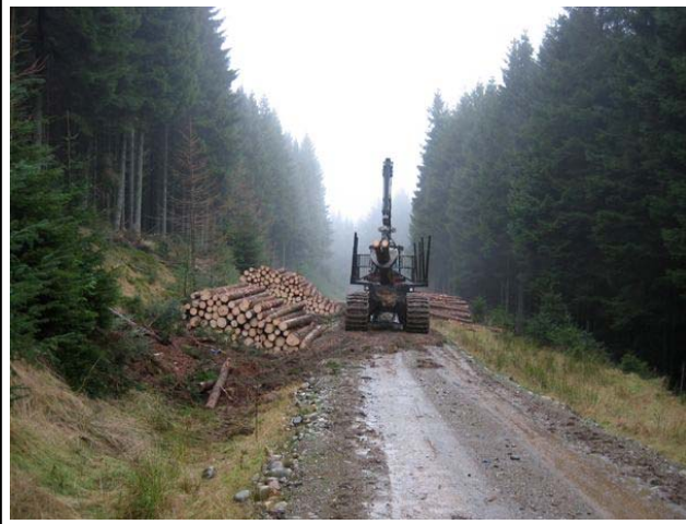
Figure 54 Forwarder timber extraction at Craigvinean (Valmet 840 fitted with full bandtracks, front and rear)
