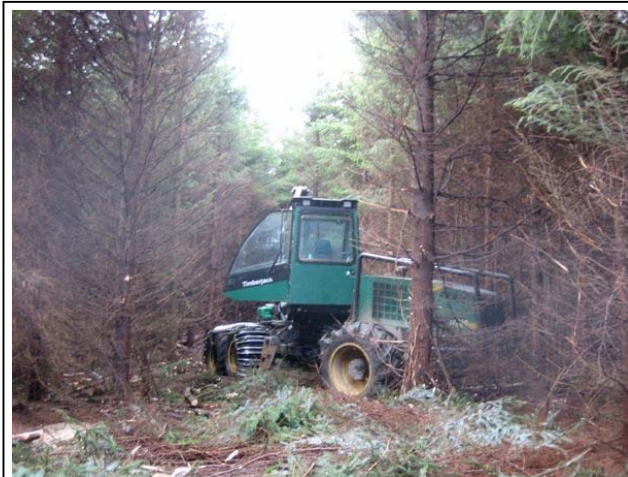
Figure 23 Timberjack 1270D harvester operating in first thinning crop
