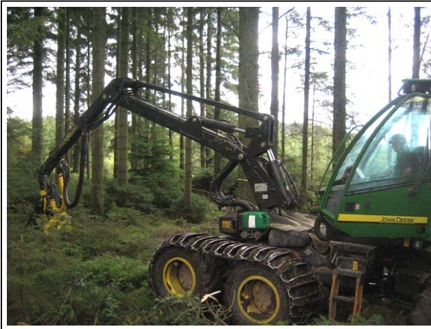
Figure 3 John Deere 1270D harvester used for felling
