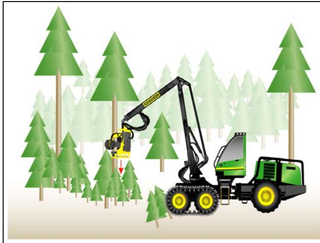
Figure 7 Locating the felling head high up the stem and running the rollers down to the base to accurately locate the felling cut in dense regeneration
