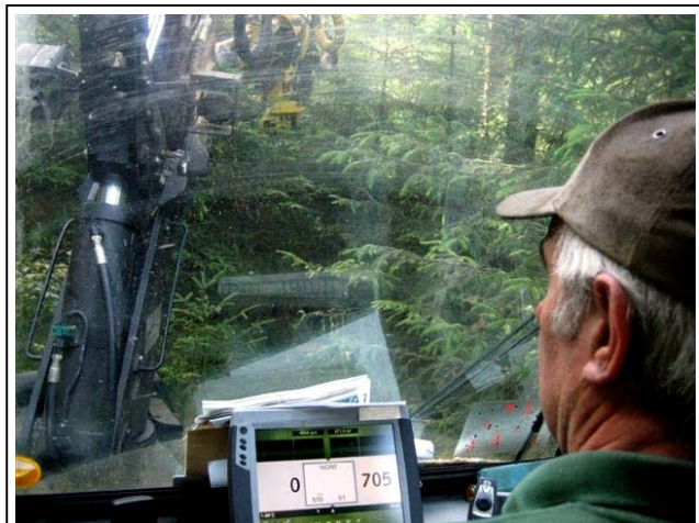
Figure 6 Restricted operator visibility from the harvester cab
