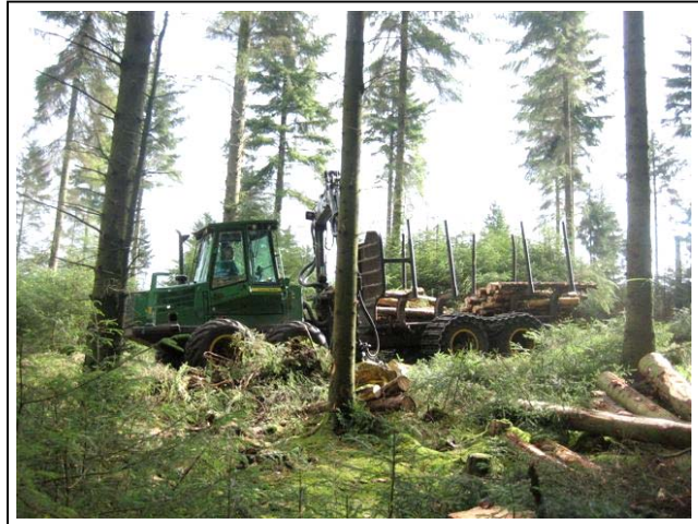
Figure 4 Forwarder extraction with John Deere 1110D
