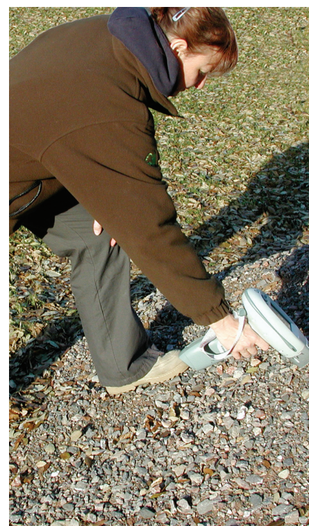
Figure 1 On-site analysis of heavy metals in a spoil heap.
