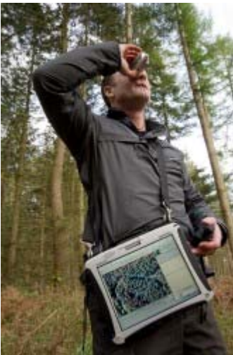
Figure 12. A surveyor measures a tree's height using an electronic vertex hypsometer.
