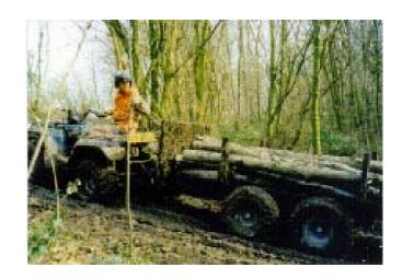
attainable. Extracting over a distance of 100 m, output should be above 2.0 m³/shr. This gives an extraction cost of £5.30/m³ and when felling is included the total system cost is £13.30/m³ assuming a felling output of 1.12 m³/shr. Use of marginal costs can reduce extraction output cost to £1.00/m³.
