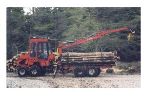
However, these units do not have the same low impact on terrain and may not have the manoeuvring ability of purpose built mini forwarders.
