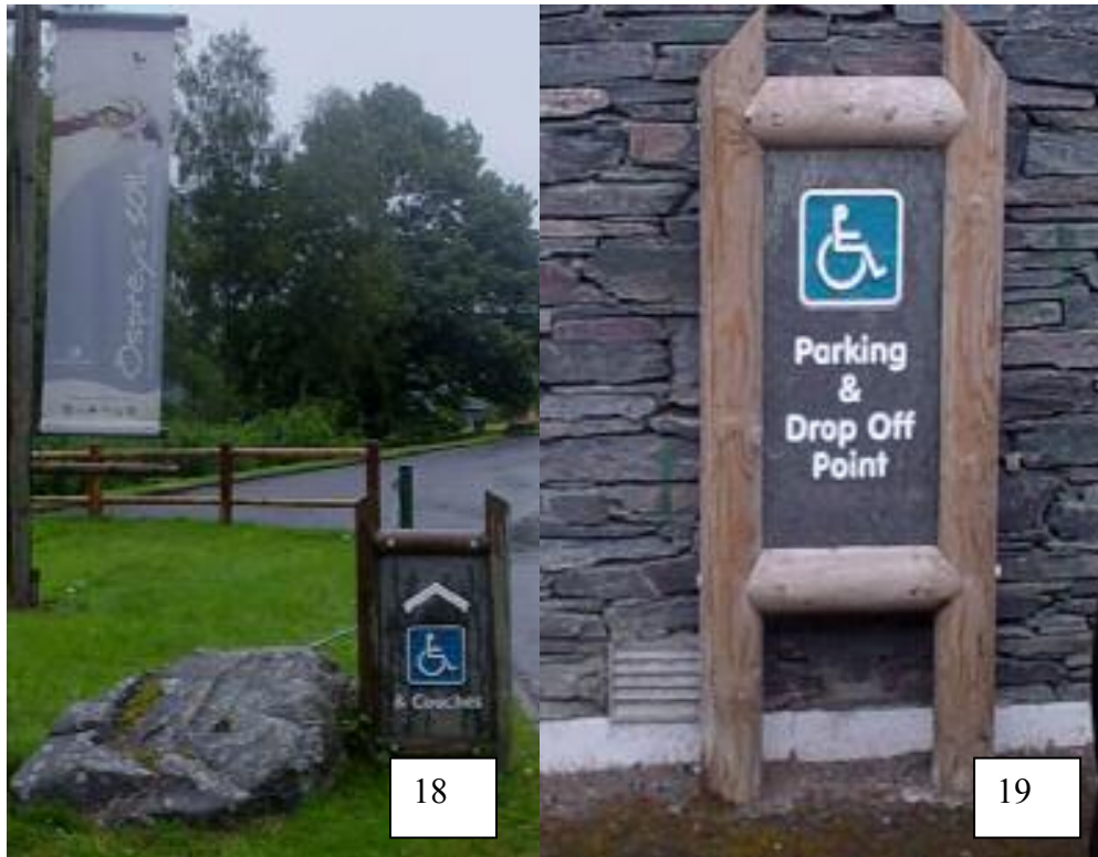
Fig 18 & 19, provision for disabled parking clearly indicated at entrance, but signage obscured at arrival point owing to low level siting.
