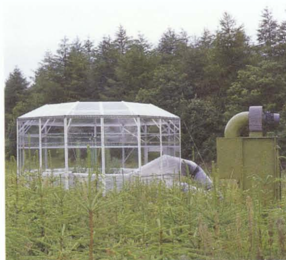
Figure 3. An open-top chamber. (40244). Air is blown through filters in the cabinet to control air quality and is then distributed around the chamber through the polythene tube before being expelled through the open top.
