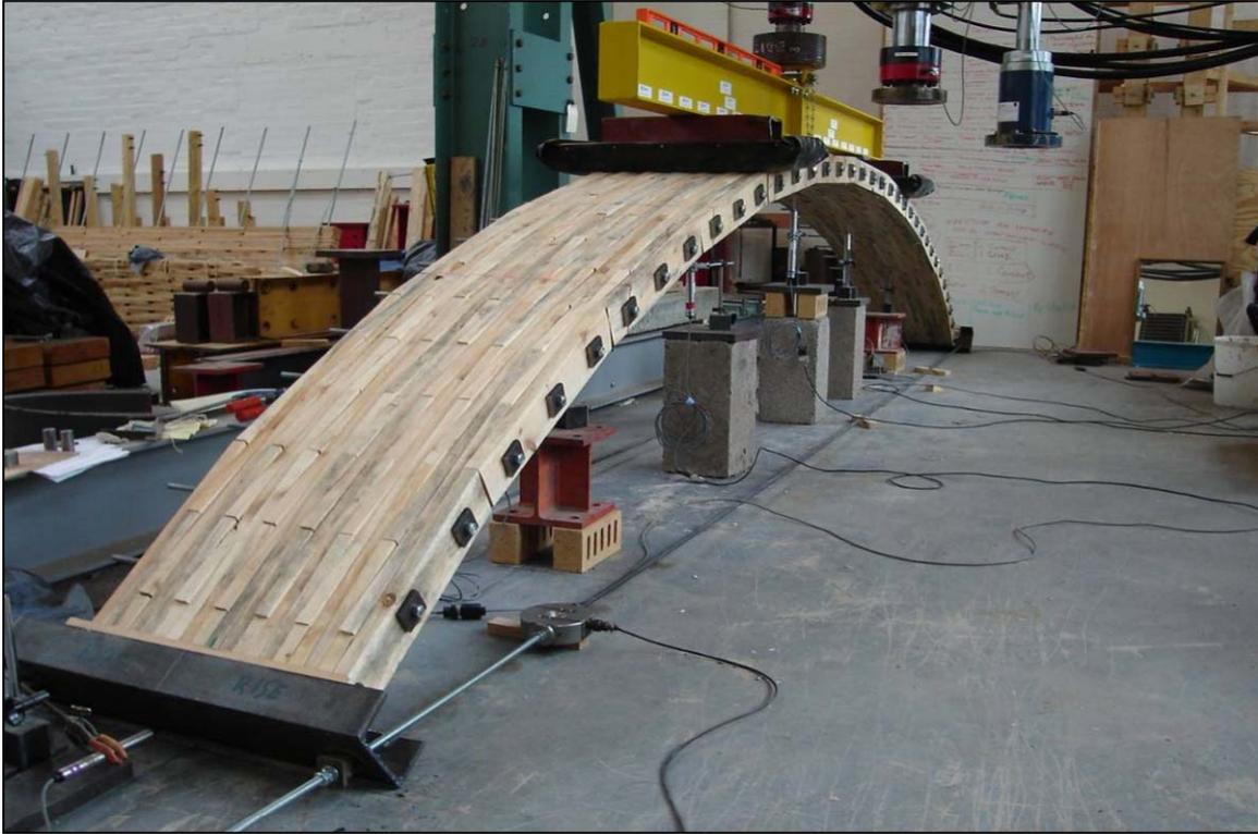
Fig 4. A stress laminated bridge being tested at Napier University
