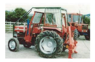
Winching can be done from the extraction routes, which can be relatively far apart (30 m to 50 m). Less area is taken up by such extraction routes than by those for a farm tractor equipped with hydraulic grapple loader and bogie trailer system.
