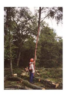
The telescopic pole is split into three 2 m sections giving a full reach of over 6 m when fully extended. A knuckle joint at the top of the telescopic shaft allows the saw bar to be adjusted against the branch being cut. Chain lubrication is from the hydraulic supply to the motor at the top of the pole.
