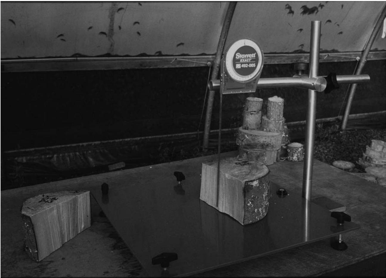
**Figure 2:** Measurement of grain angle
