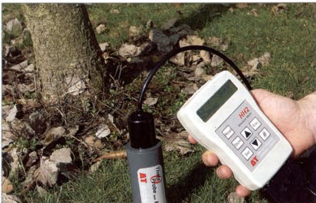
Fig. 1: soil moisture content being measured using a Delta-T Devices Theta probe and moisture meter
