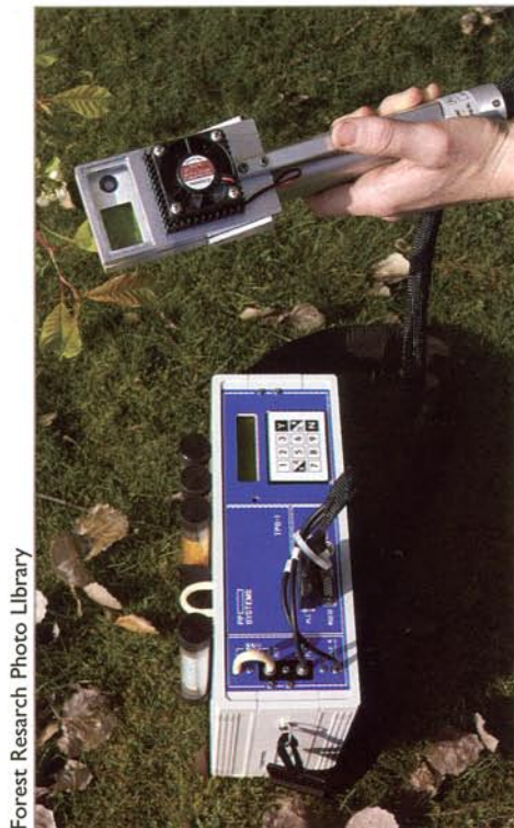
Fig 2: PP-Systems CIRAS-1 infra-red gas analyser and leaf chamber
