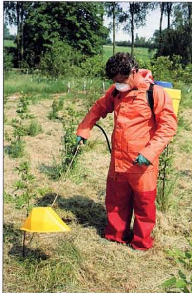
Forestry spot gun (right) Adapted drenchgun with a lighter 5 litre knapsack, delivering a 5 ml measured dose.
