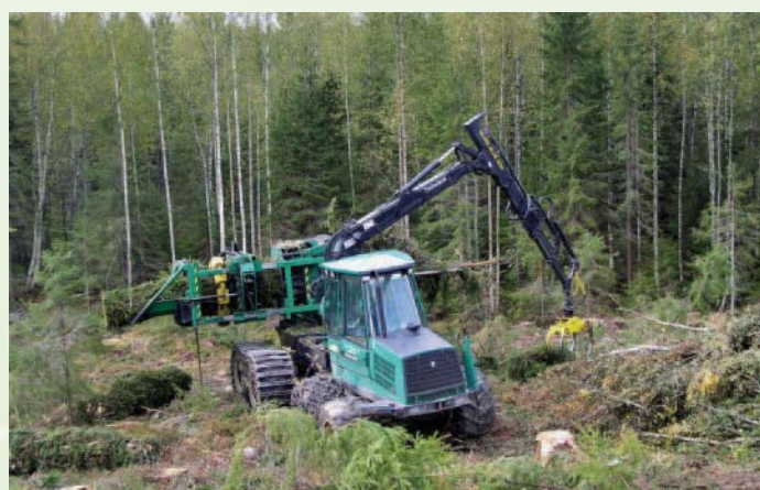
Producing bales from branchwood left over from tree felling at a scale suited to large-scale woodfuel energy production
