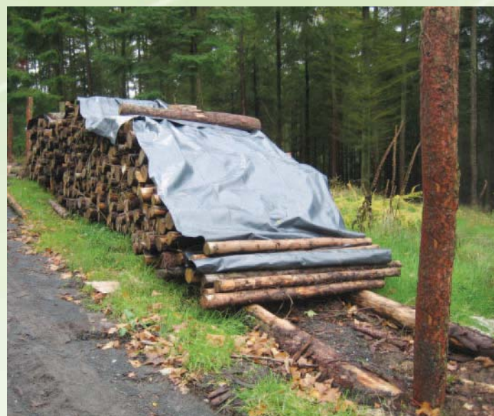
Timber stack organised into a corral, showing logs stacked on bearers and covered with impermeable sheeting to prevent re-wetting
