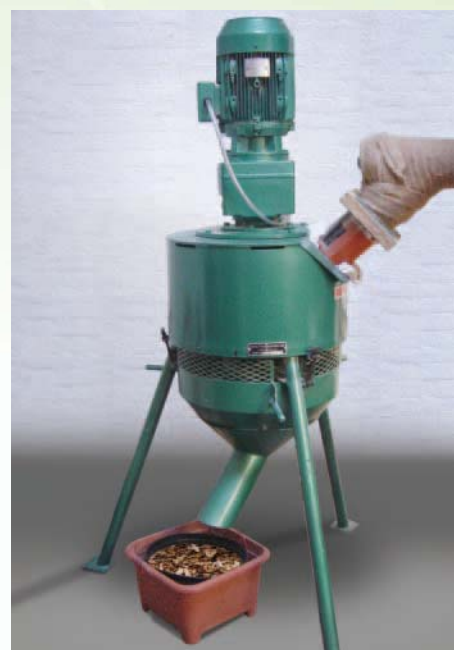
Small-scale wood pelletiser unit used to produce wood pellets for fuel
