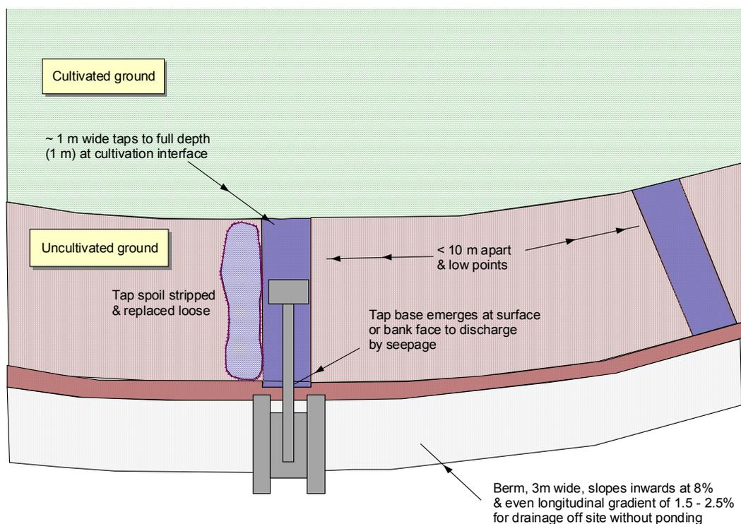
**Figure 8.** Drainage tap plan (example meets drainage berm)
