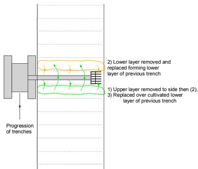
**Figure 5.** Partial inversion by the side strip method
