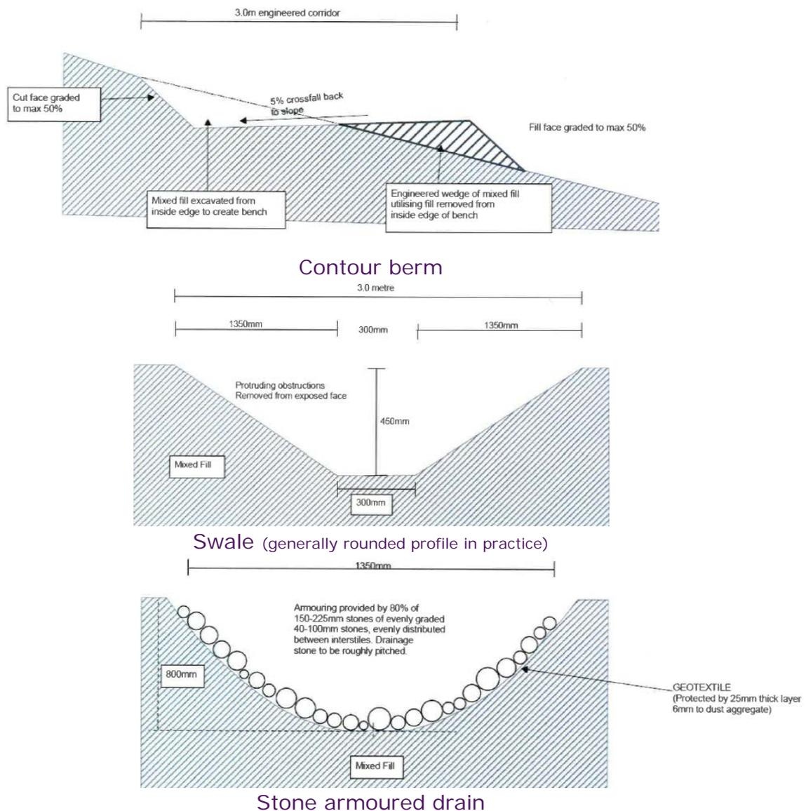
**Figure 12.** Contour berm, Swale and Armoured drain<sup>7</sup>
