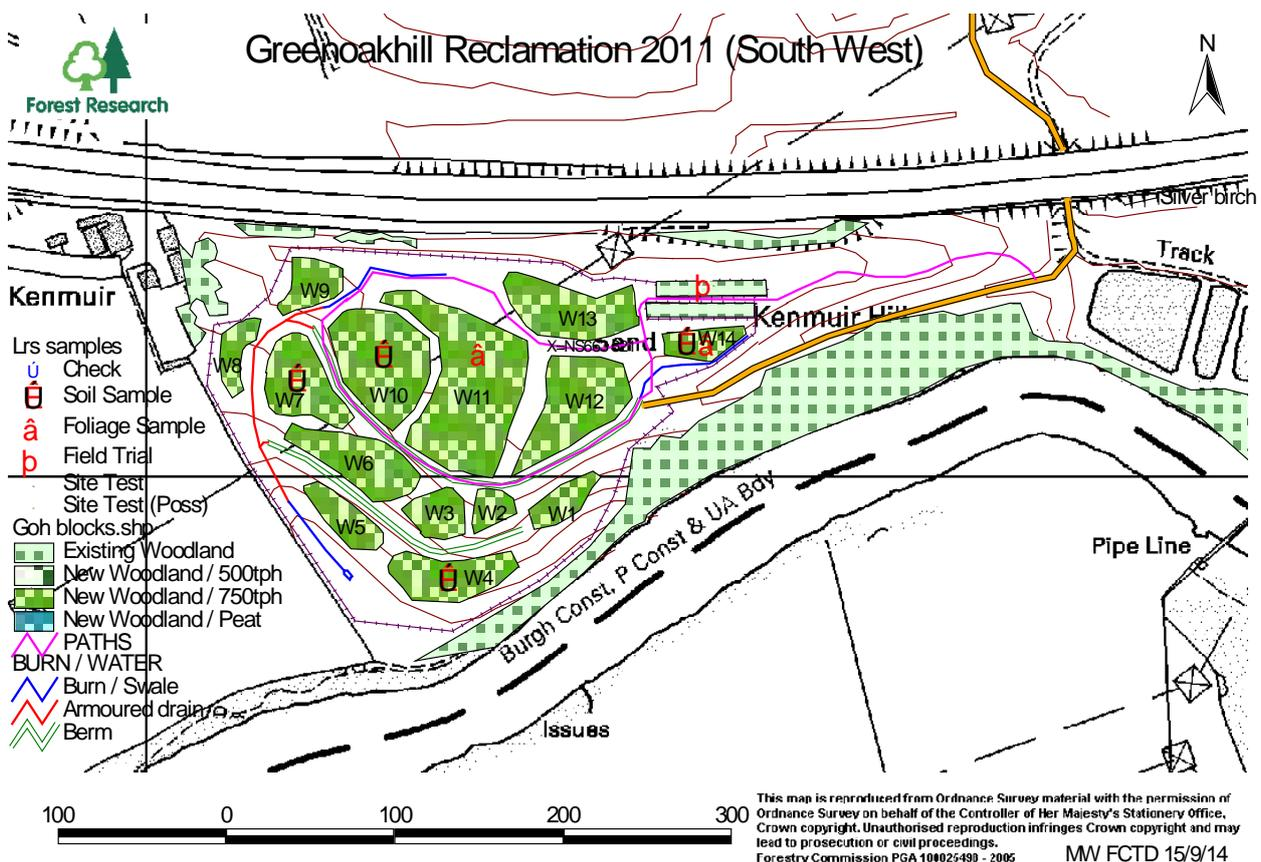
**Figure 7.** South West block completed design
