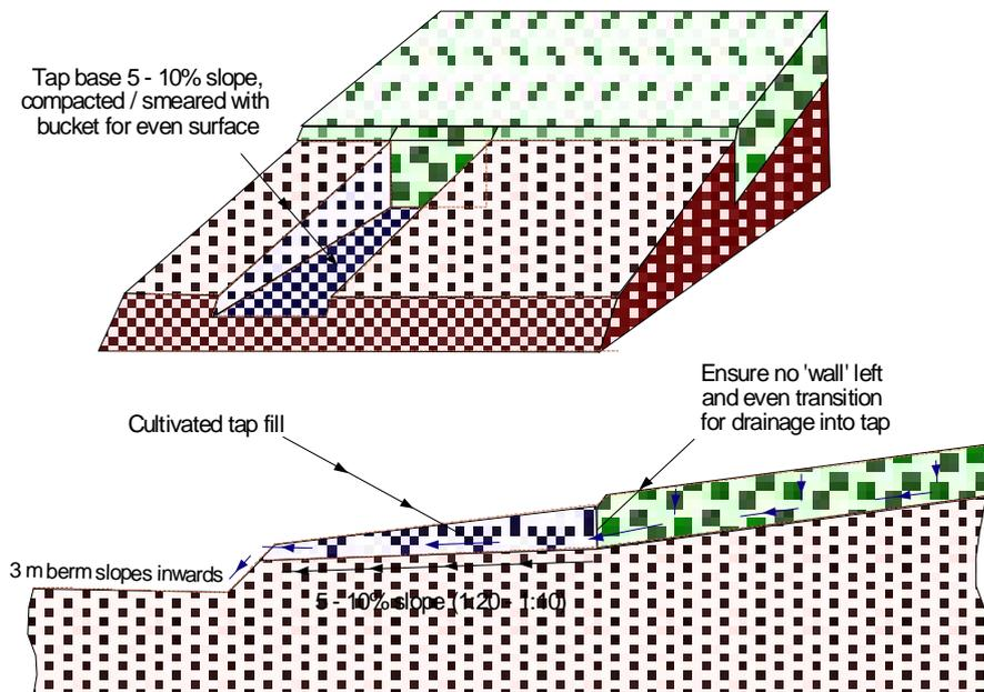
**Figure 10.** Drainage tap (meeting drainage berm). Top: view prior to loose infill
