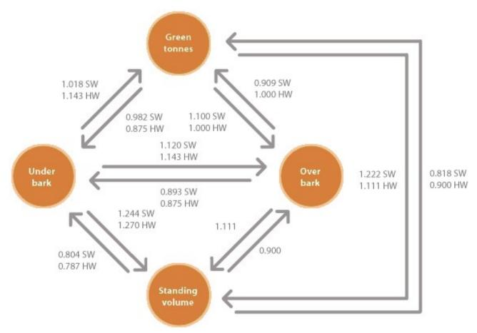
The diagram shows separate conversion factors to use when converting softwood (SW) and hardwood (HW) with arrows to indicate the direction of conversion. For example, to convert 1,000 green tonnes of SW into an under bark volume, the 1,000 green tonnes should be multiplied by the conversion factor of 0.982 to give 982m³ underbark. There is no difference between the softwood and hardwood conversion factors for converting between standing volume and overbark volumes.
