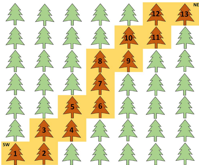
Figure 2. Standard survey method whereby thirteen trees in the order numbered were assessed per plot by moving from the south-west (SW) to the north-east (NE) corners of each plot
