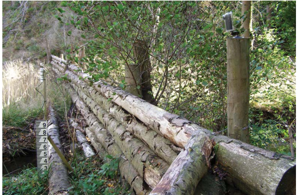
Figure 25 A camera and gauge board are used here to record how the timber dam affects high flows.
