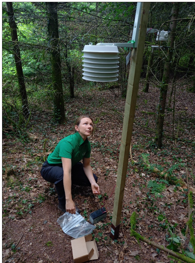
Figure 6. Setup of rotor arm trap and data logger for the monitoring of temperature and humidity at The Cott, Devauden; the data logger is enclosed in a white radiation screen to shield it from rain and direct solar radiation. The rotor arm trap is powered by a 12V battery.
