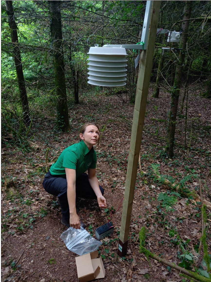
Figure 2: Setup of rotor arm trap and data logger for the monitoring of temperature and humidity at a WPHSN site. The data logger is enclosed in a white radiation screen to shield it from rain and direct solar radiation and the rotor arm trap is powered by a 12V battery..
