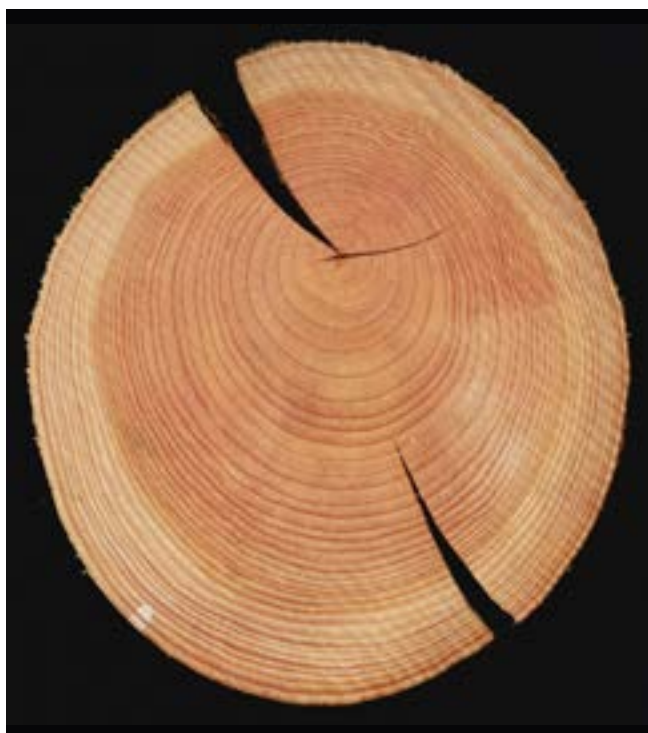
Figure 14 The lighter (outer) sapwood contrasts markedly with the darker (inner) heartwood in this disc taken from a mature Japanese larch tree.
