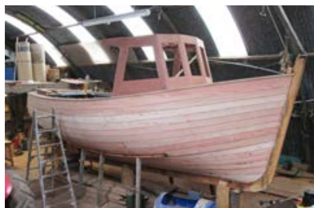
Figure 26 Boatbuilding: boat-skin larch is used where skippers still specify wooden hulls for their fishing boats, such as this one at Isle Ewe Boats, Aultbea.
