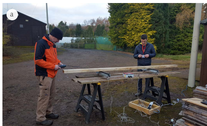
Figure 2 (a) Testing structural-sized battens using a handheld MTG timber grading machine; (b) structural-sized battens being loaded into the kiln at Forest Research's Northern Research Station for drying; (c) grand fir logs being cut on the Woodmizer sawmill; (d) sycamore logs being marked with cutting pattern prior to cutting.
