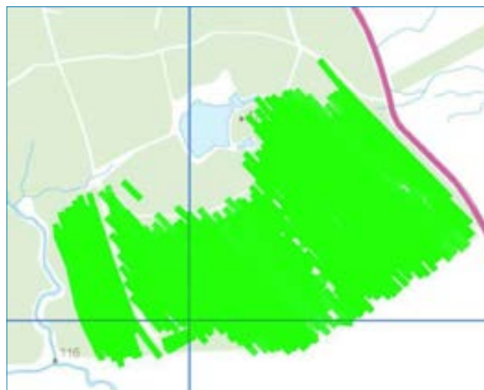
Figure 10 This spread pattern recorded by a helicopter guidance system shows that the use of map coordinates to guide aerial fertiliser application can reduce the risk of treating buffer areas.
