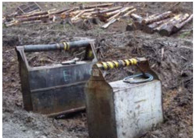
Figure 31 Containers placed on uneven ground are more liable to tip over, resulting in serious spillage.
