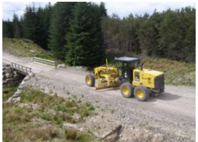
Figure 17 Careful planning and execution of construction and maintenance work is key to minimising the threat of sediment pollution.
