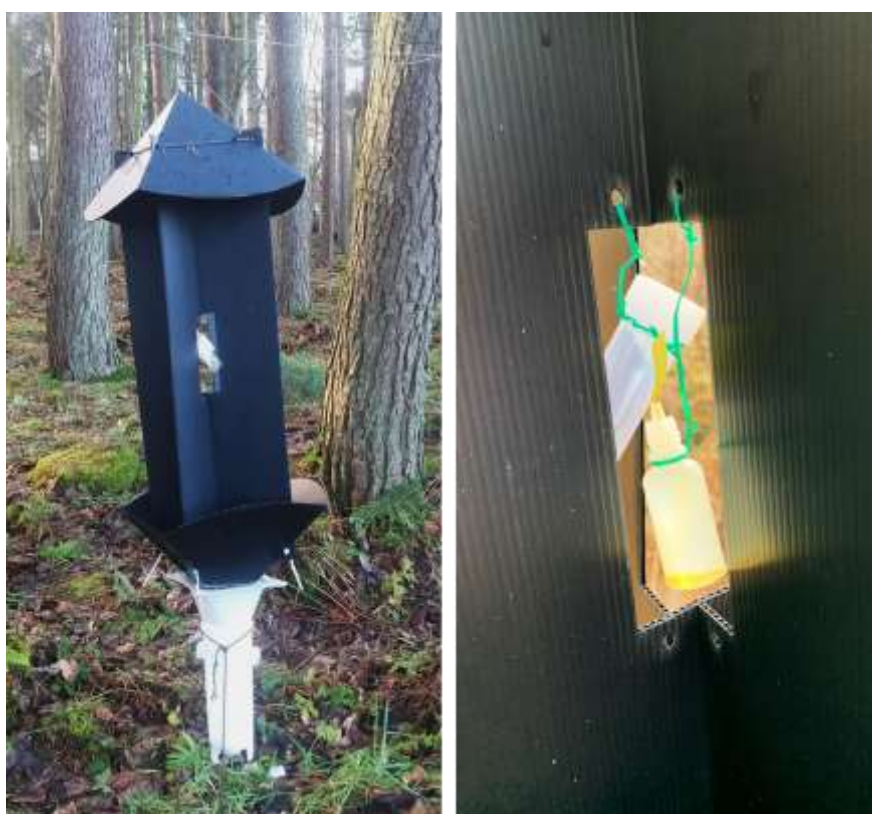
Fig. 2. Set up of a typical cross-vane trap (left). Ethanol and alpha-pinene lures in place in a cross-vane trap (right).
