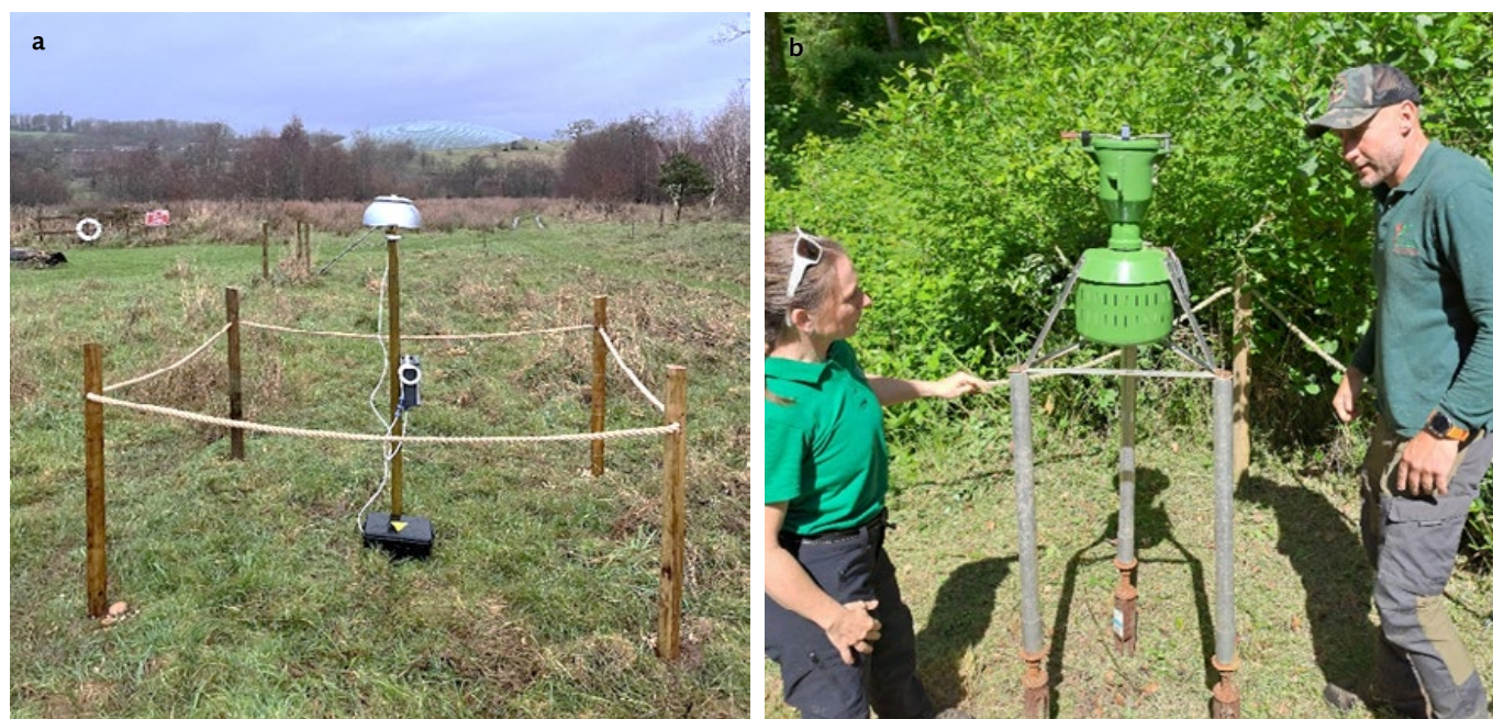
Figure 7 Air samplers used for 2025 spore surveillance: a) Agri Samplers™ Rotorod sampler; b) Burkard™ 7-day sampler.
